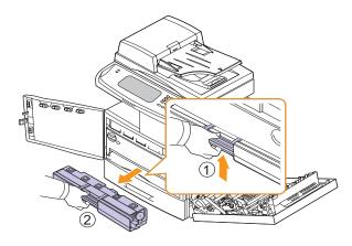
Turn the imaging unit locking levers outwards to release and open the inner cover.
